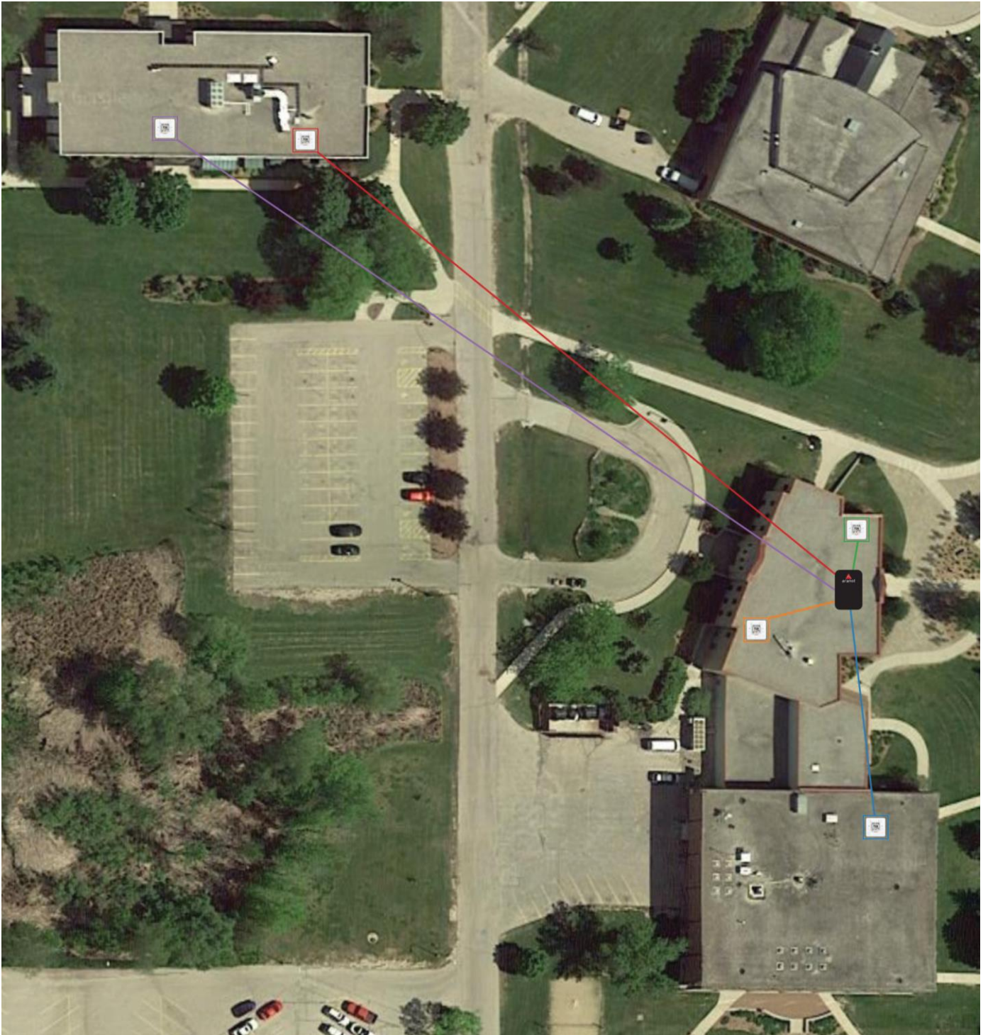
Figure 1: Lakeland University Aerial Map w/ Aranet4 PRO sensors & Aranet PRO base station.
